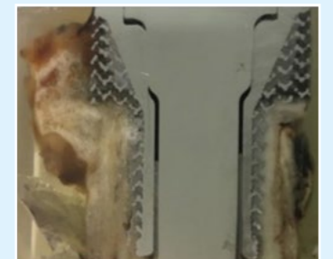
Fig 3. Cross section of a retrieved collar demonstrating the amount of bone ingrowth throughout the porous structure.
